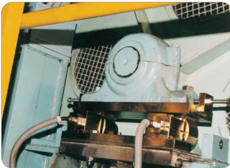
In web tension measurement, the cylindrical shape means that the load cell can be rotated in its mounting so that it measures the resultant force.
